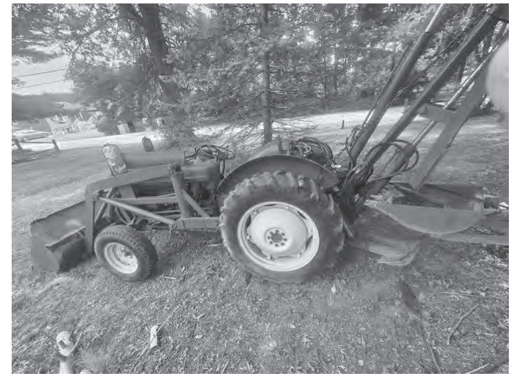
Courtesy photos This is a Wain Roy backhoe attached to a Ford tractor.
