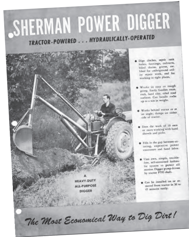
This shows an ad for the Wain Roy/Sherman power digger. The digger or backhoe attached to a tractor and operated with hydraulics.
